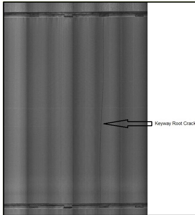
Figure 3 – Keyway Root Crack Example
