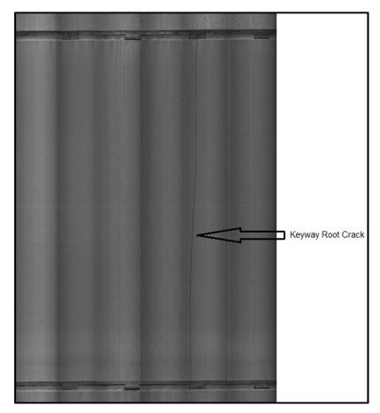
Figure 3 – Keyway Root Crack Example
