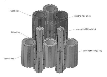
Figure 1 – Graphite Core Arrangement
