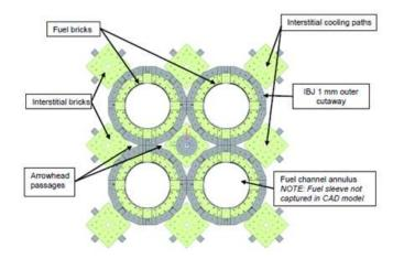
Figure 4 – Plan view of graphite core showing arrowhead passages, and annulus with no fuel stringer in-situ
