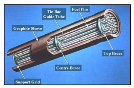
Figure 2 – Fuel Element Example
