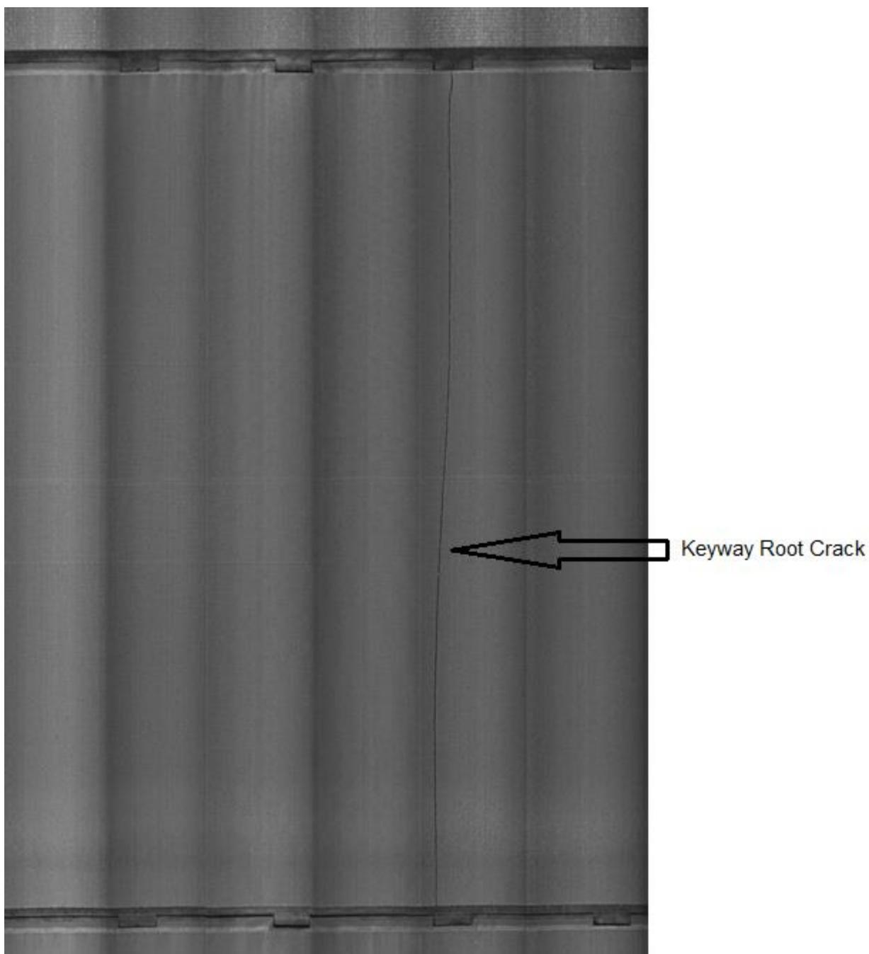
Figure 3 – Keyway Root Crack
