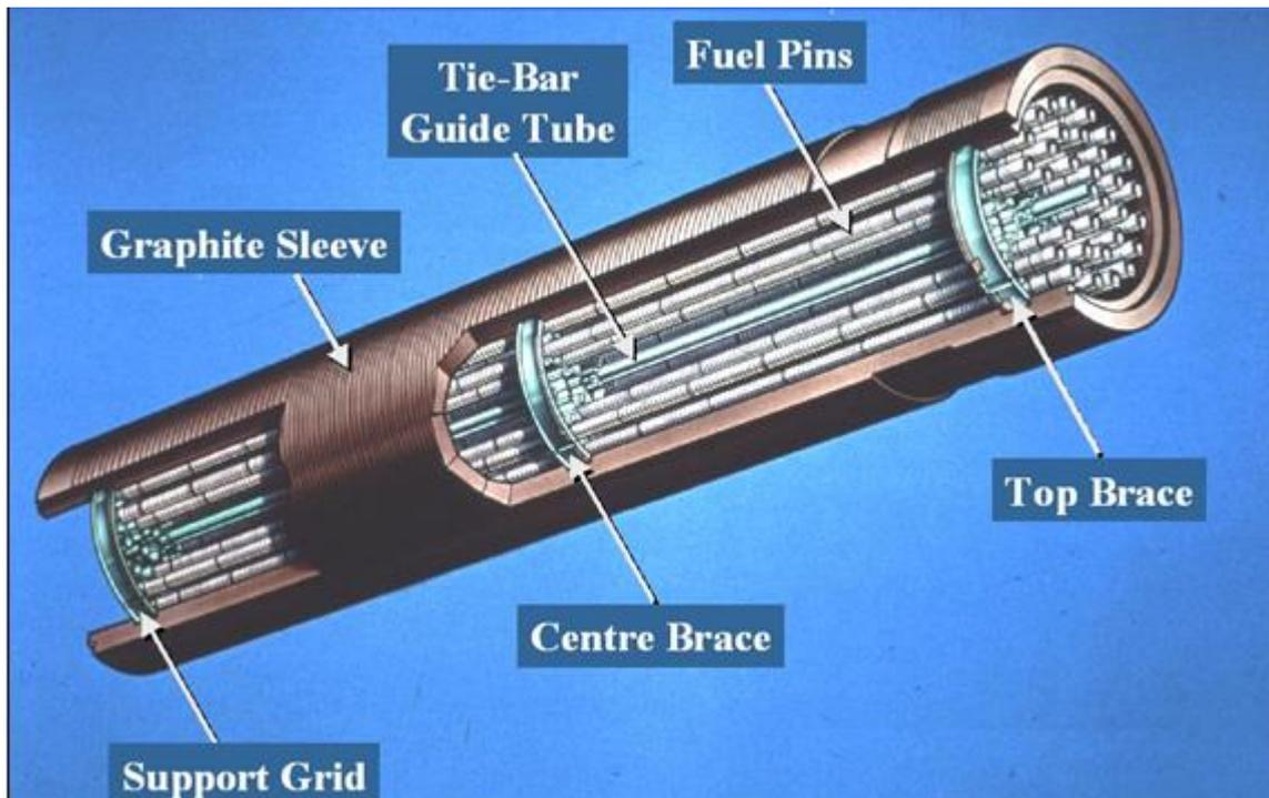
Figure 2 – Fuel Element Example
