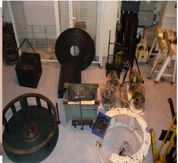
Photograph 3c – Some attempt to store components but with little or no traceability and a mixture of different plant items.
