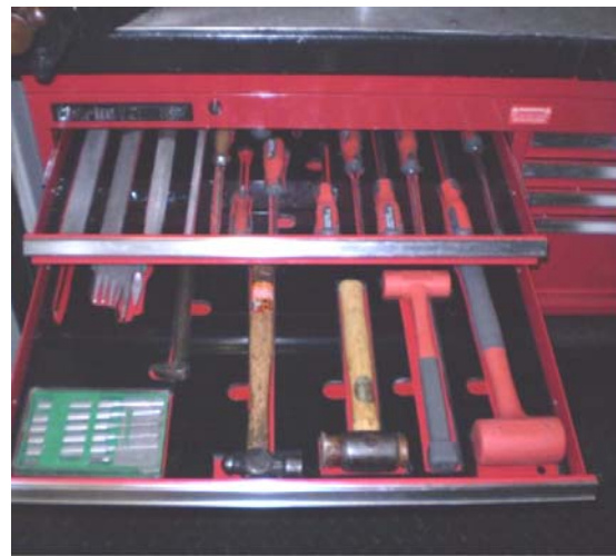
Photograph 1B – Good practice where each tool has designated storage locations.
