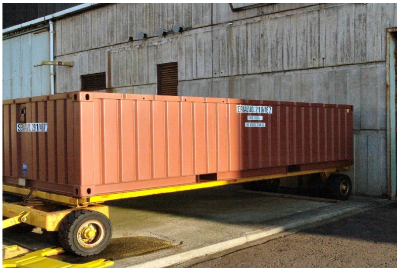
Photograph 2 - Example of a half-height ISO container awaiting transport from a Magnox Ltd site to the LLW Repository
