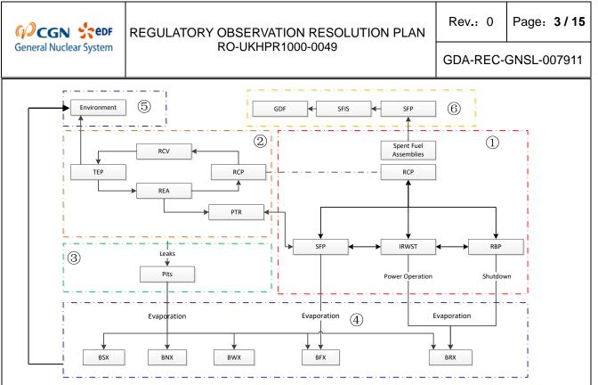
Fig 1 The Diagram of the Whole Process of Tritium Transport
