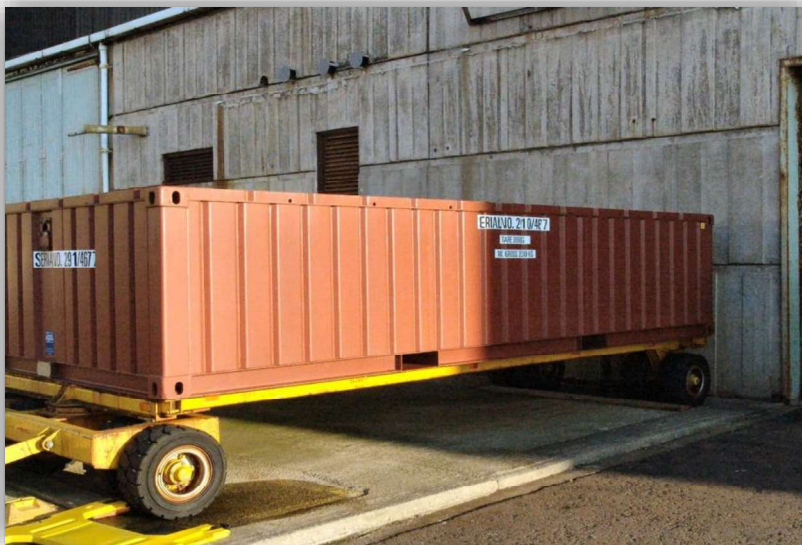
Photograph 2 - Example of a half-height ISO container awaiting transport from a Nuclear Restoration Services site to the LLW Repository
