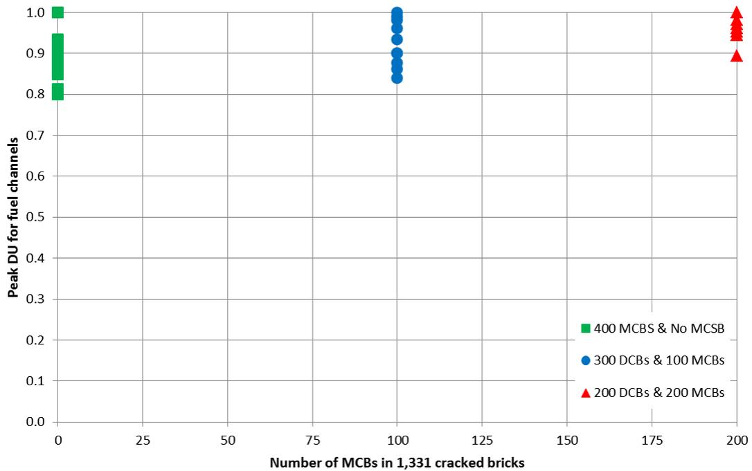
Figure 7: Fuel channel peak DUs for normal operation, SCBs, DCBs and MCBs.
