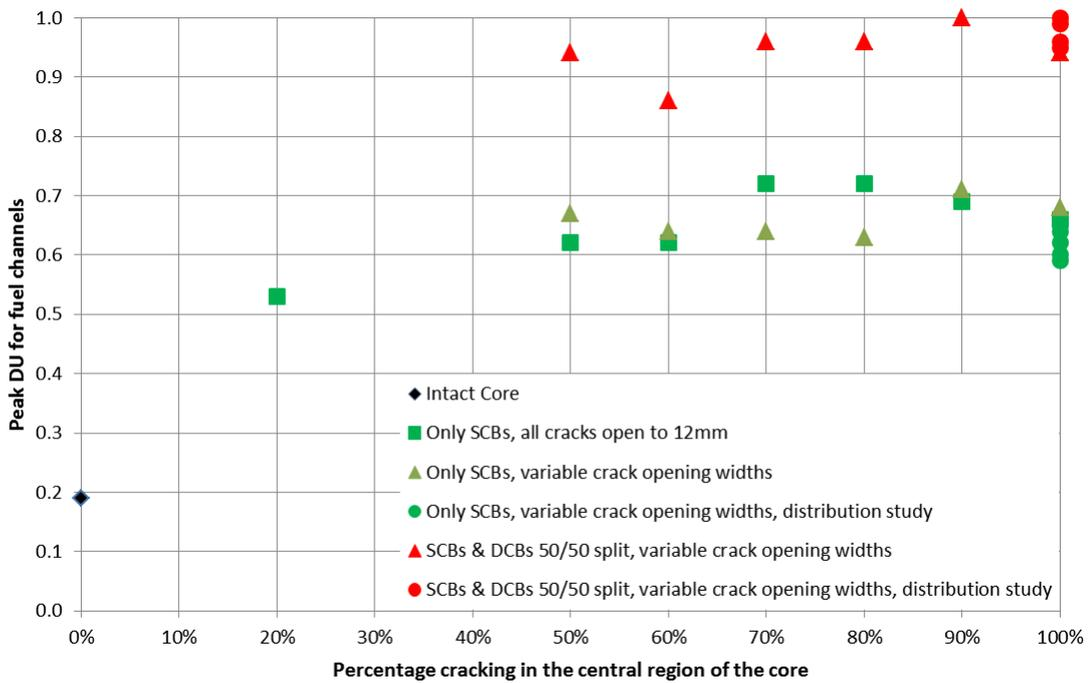
Figure 5: Fuel channel peak DUs for normal operation, SCBs and DCBs only.
