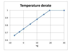
152. At 0°, the 1-minute rate battery capacity is typically 75% of nominal for Nickel-Cadmium cells. However, there is a compounding effect: the larger the discharge current in relation to the capacity, the less Amp-hours are available.
