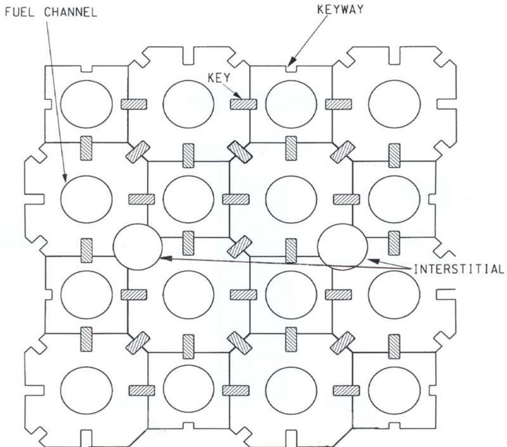
Figure 2 - Plan Arrangement of Wylfa Graphite Bricks
