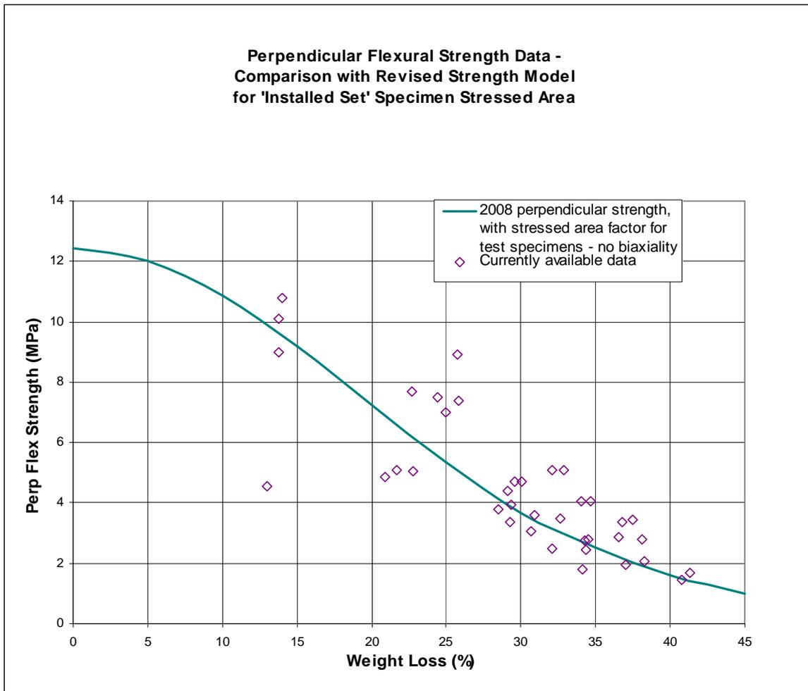
Figure 3: Comparison of the Emergent 'Installed-Set' Perpendicular Flexural Strength Data for the Test Specimens and the Strength Relationship Employed.
