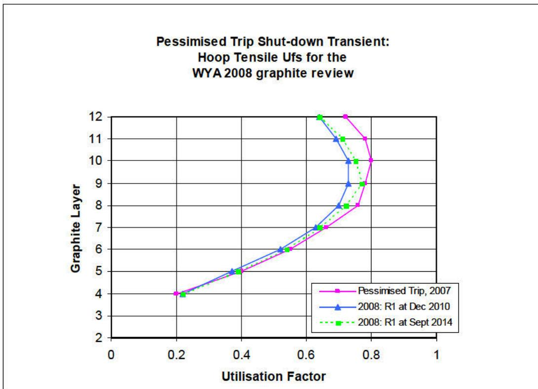
Figure 5 (b) Shut-down Transient FCW Hoop Tensile Utilisations
