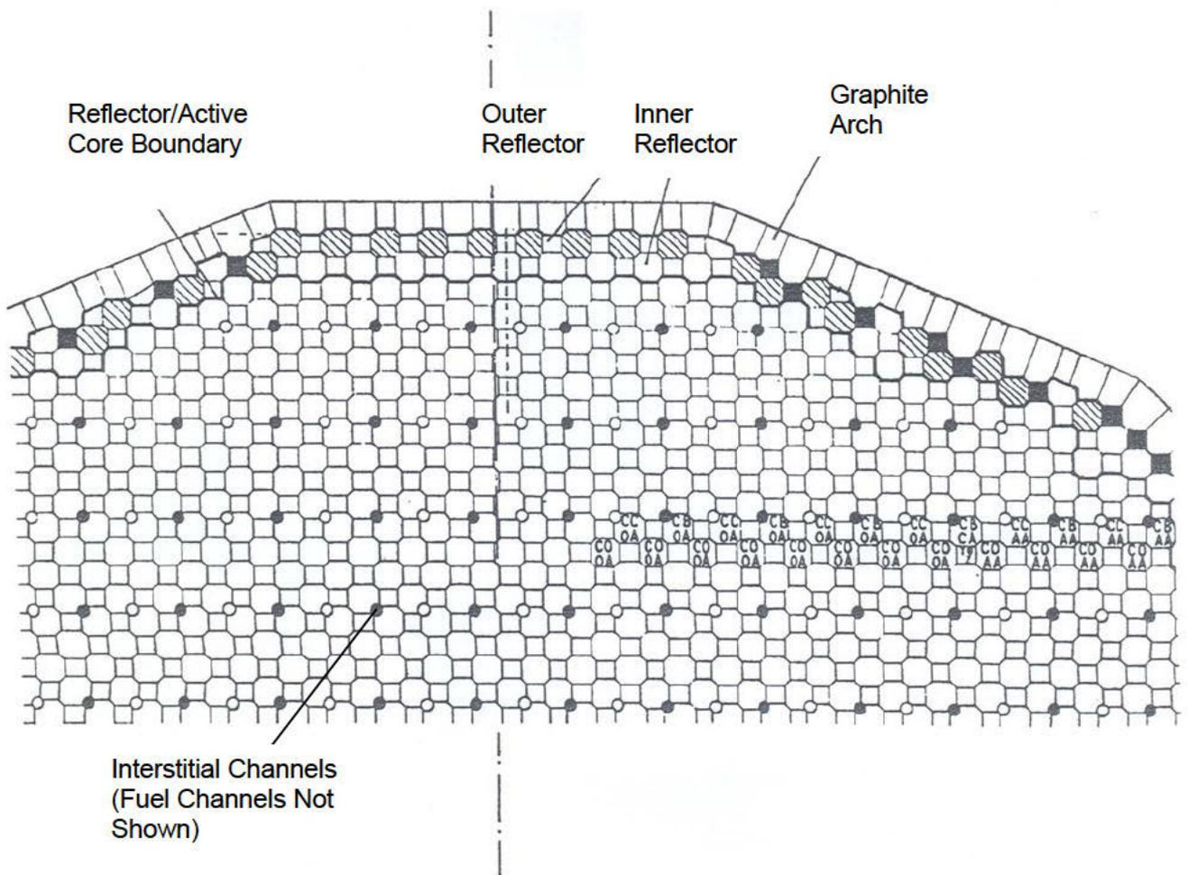
Figure 1 – Plan View of Wylfa Graphite Core Showing Graphite Arch and Reflector
