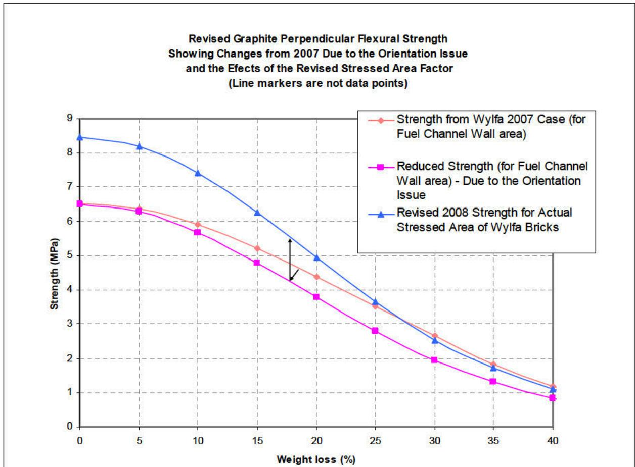
The revised strength relationship has a stressed area factor defined as  $a^{-0.0555}$  where  $a$  is the stressed area in  $\text{mm}^2$ . The fuel channel wall area is  $247000\text{mm}^2$ ; for octagonal bricks, the FEAT model calculates a  $a$  as  $2000\text{mm}^2$ . A biaxiality factor of 0.8 is applied throughout.
