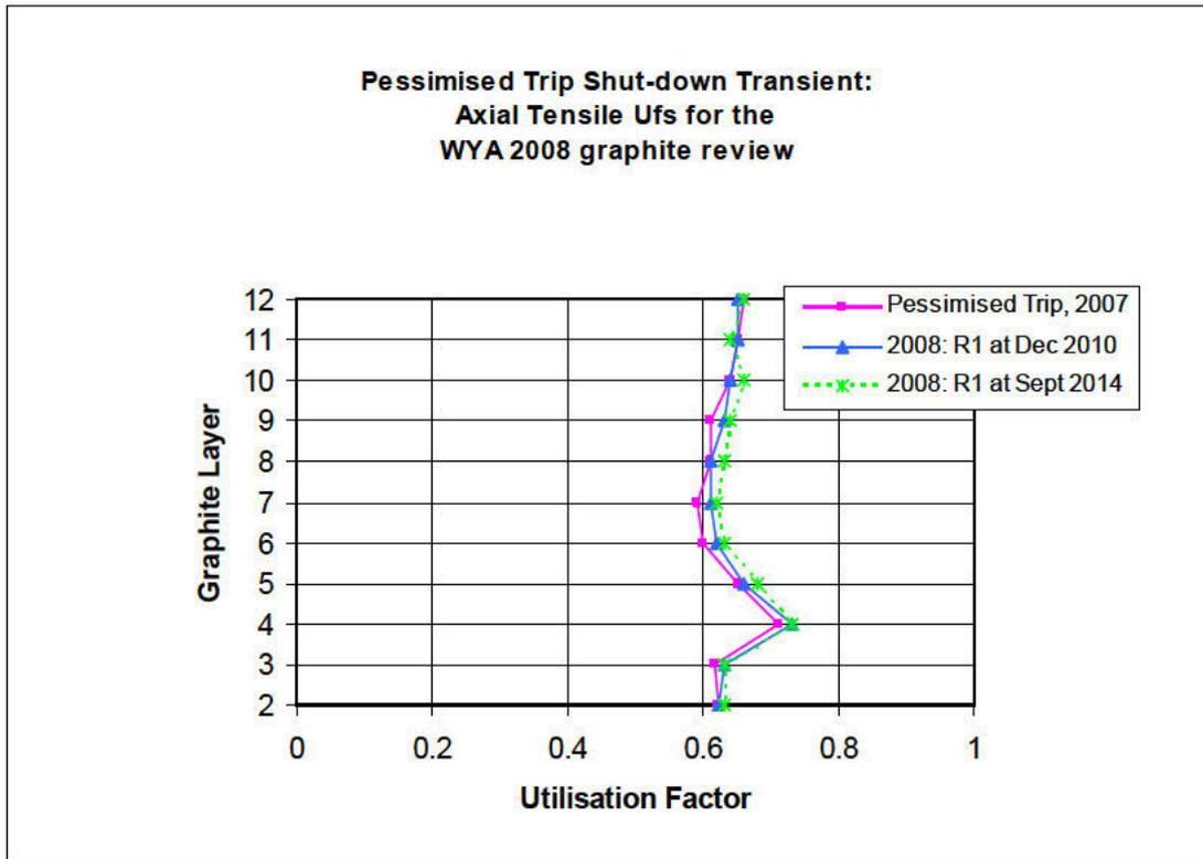
Figure 5 (a) Shut-down Transient FCW Axial Tensile Utilisations – Note that the biaxiality factor is removed from the strength for Graphite layers 2 and 3 due the absence of significant hoop stress
