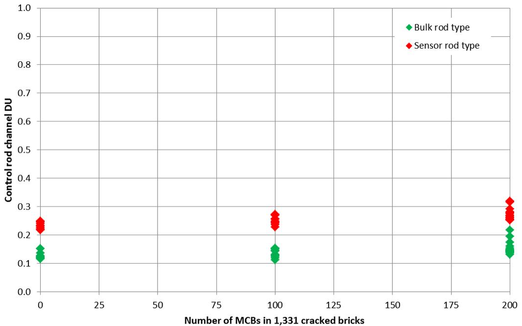
Figure 12: Control rod channel peak DUs for seismic, SCBs, DCBs and MCBs.
