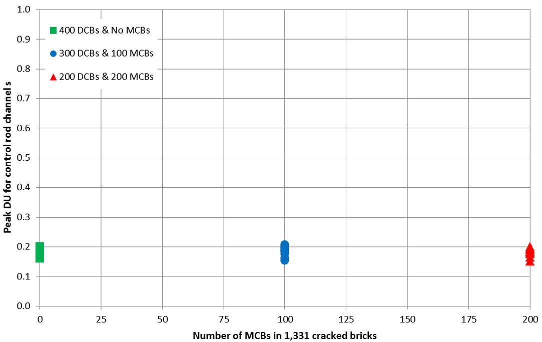
Figure 6: Control rod channel peak DUs for normal operation, SCBs, DCBs and MCBs.
