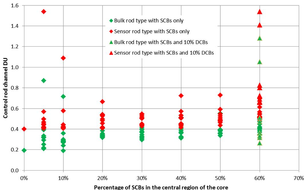
Figure 9: Control rod channel peak DUs for seismic, SCBs and DCBs only.
