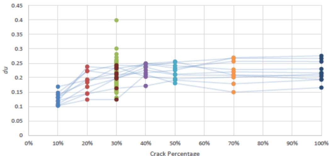
Figure 8: DU variation for different levels of cracking and random distributions. (Taken from Reference 67, at 30% there are 64 different random distributions evaluated, at all other percentages there are 10.)
