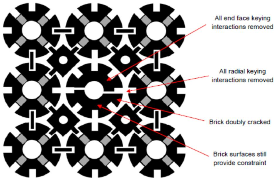
Figure 3: Representation of Multiply-Cracked Fuel Brick (Proxy-MCB).
