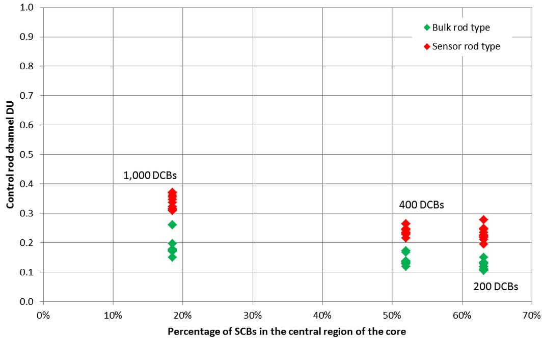
Figure 11: Control rod channel peak DUs for seismic, updated PCPV model.
