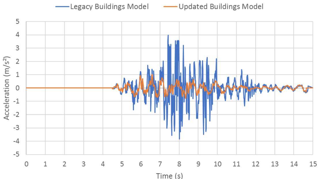
Figure 10: Legacy and revised seismic input to the graphite core.
