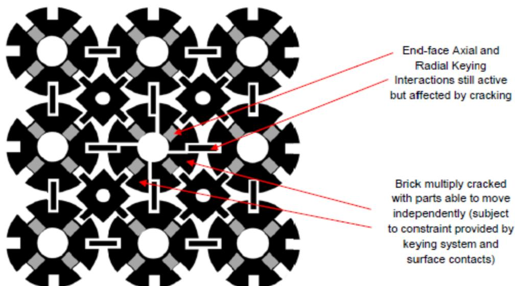
Figure 2: Potential Multiply-Cracked (Quadruple-Cracked) Fuel Brick.
