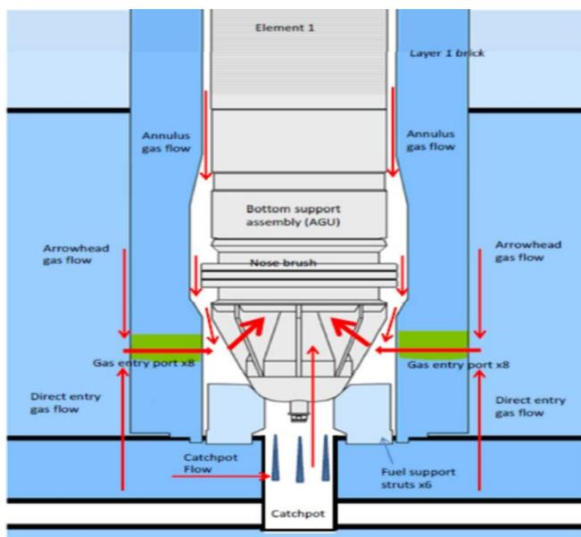
Figure 16: Illustrative flow paths at the base of the fuel channel for HPB/HNB.
