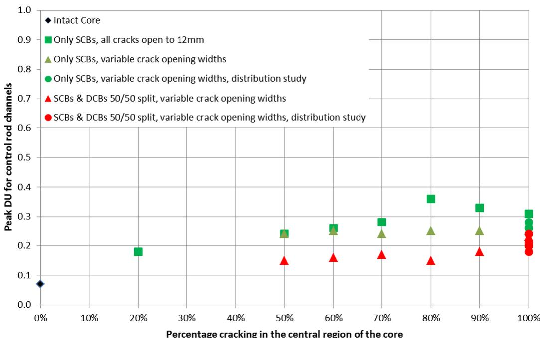
Figure 4: Control rod channel peak DUs for normal operation, SCBs and DCBs only.
