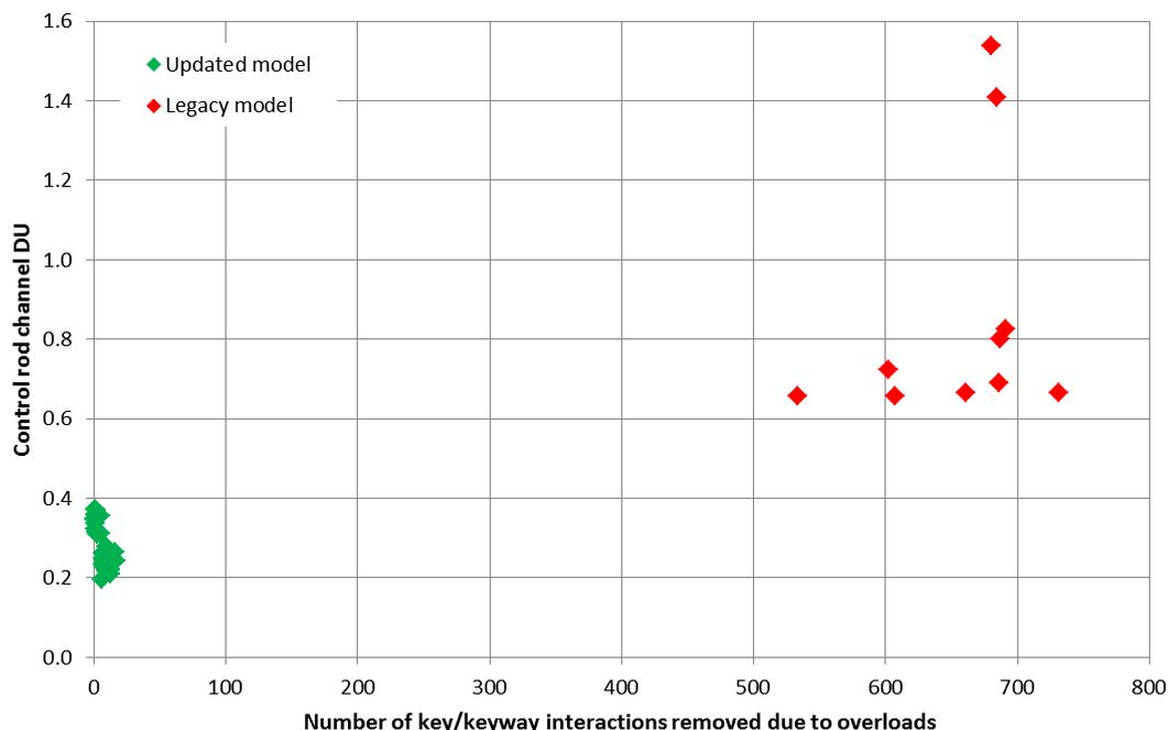
Figure 13: Correlation of peak DUs to keying system failures.
