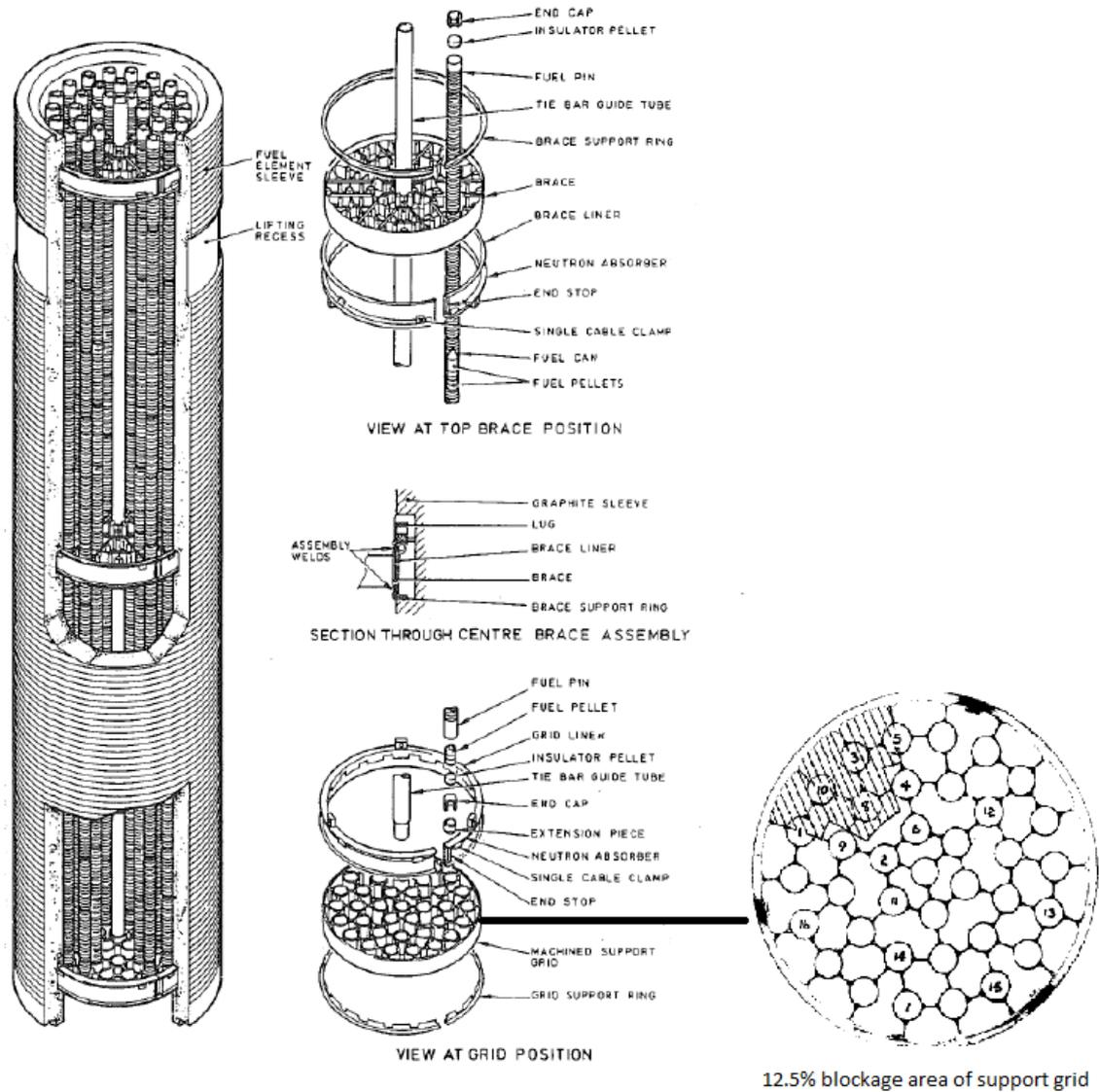
Figure 15: Illustration of an AGR fuel element.
