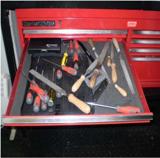
Photograph 1a –Poor Practice for storing tools in a cabinet
