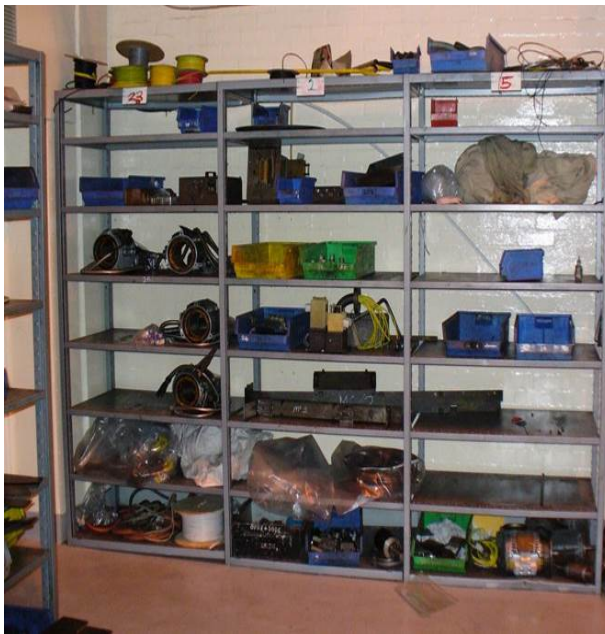
Photograph 3c – Some attempt to store components but with little or no traceability and a mixture of different plant items.
